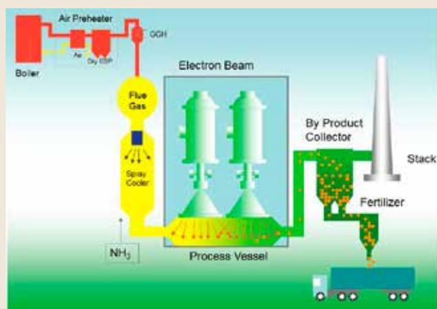
Scheme of the electron beam flue gas treatment (not to scale).
