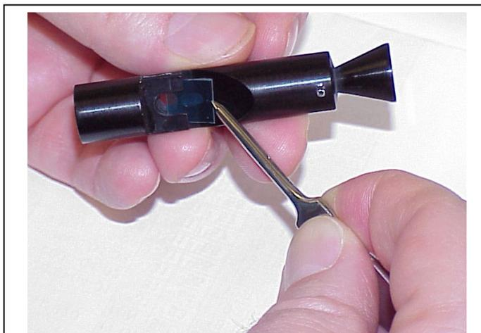
*Photograph 2: A pair of fine pointed tweezers is being used to hold the dosimeter film along one edge whilst placing it inside the reader dosimeter holder. Notice that the tweezers touch only the edge of the film to avoid scratching the centre of the film where the OD reading will be taken.*
