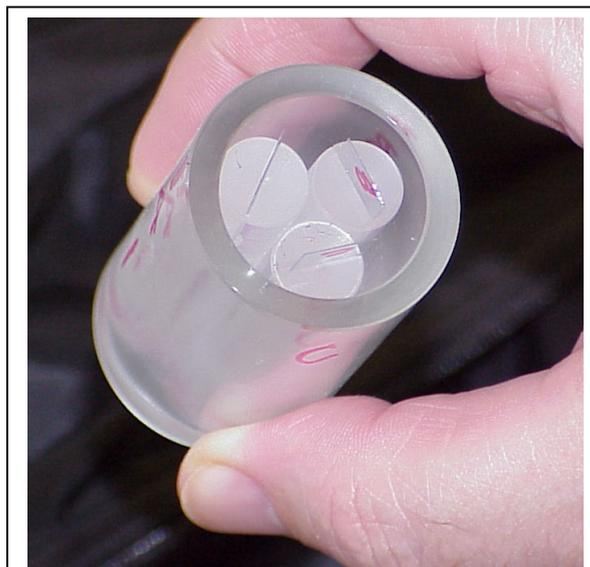
Photograph 6: Three film holders with Gafchromic® dosimeters are placed in a cylindrical holder for irradiation in a Gammacell. Note that each film holder is placed so that the film is parallel (tangential) to the curved surface of the dosimeter holder. For a flat dosimeter holder, the film holders should be placed so that the films are parallel to the longer face of the dosimeter holder.
