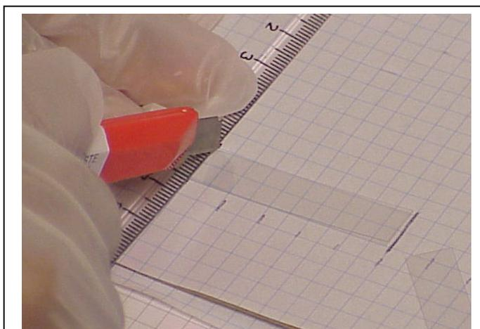
*Photograph 3: A sharp utility knife, a plastic ruler and a grid paper under the film help to cut it in desirable lengths conveniently. Apply a slight pressure on the ruler with the other hand to keep the film from moving during cutting. It is very essential that a pair of thin surgical gloves is used during this activity to avoid fingerprints.*
