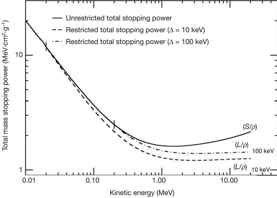
FIG. 2.2. Unrestricted  $S/\rho$  and restricted  $((L/\rho)_\Delta$  with  $\Delta = 10$  and  $100$  keV) total mass stopping powers for carbon ( $\rho = 1.70$  g/cm<sup>3</sup>), based on data published in ICRU Report No. 37. Vertical lines indicate the points at which restricted and unrestricted mass stopping powers begin to diverge as the kinetic energy increases.
