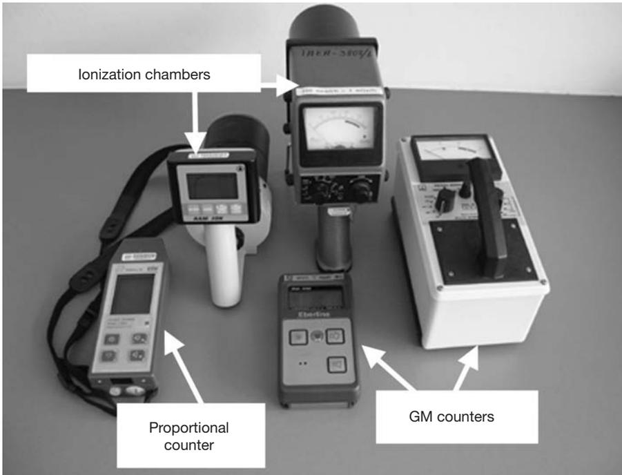
FIG. 4.2. Area survey meters commonly used for radiation protection level measurements: ionization chambers, a proportional counter and GM counters.
