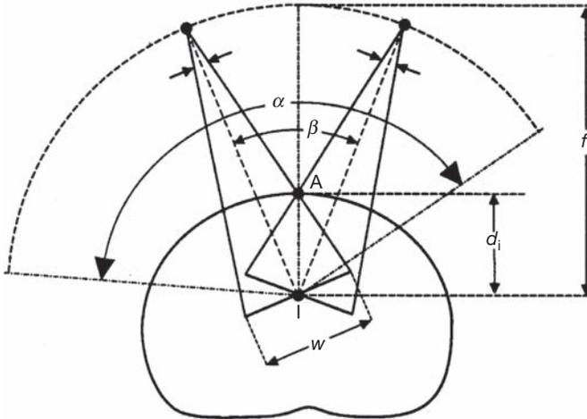
FIG. 8.10. Arc therapy geometry:  $f$  is the SAD;  $d_i$  is the depth of the isocentre;  $w$  is the field width defined at the isocentre;  $\alpha$  is the arc angle or the angle of treatment; and  $\beta$  is the characteristic angle for the particular treatment geometry.
