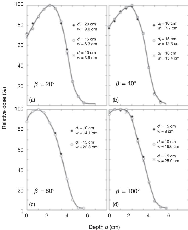
*FIG. 8.11. Radial PDDs in electron arc therapy measured in a phantom for various combinations of  $w$  and  $d_s$ , giving characteristic angles  $\beta$  of (a)  $20^\circ$ , (b)  $40^\circ$ , (c)  $80^\circ$  and (d)  $100^\circ$ . The electron beam energy is 9 MeV.*
