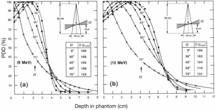
FIG. 8.5. PDD curves for various beam incidences for a (a) 9 MeV and (b) 15 MeV electron beam.  $\alpha = 0$  represents normal beam incidence. The inset shows the geometry of the experimental set-up and the doses at  $z_{max}$  for various angles  $\alpha$  relative to the dose at  $z_{max}$  for  $\alpha = 0$ .
