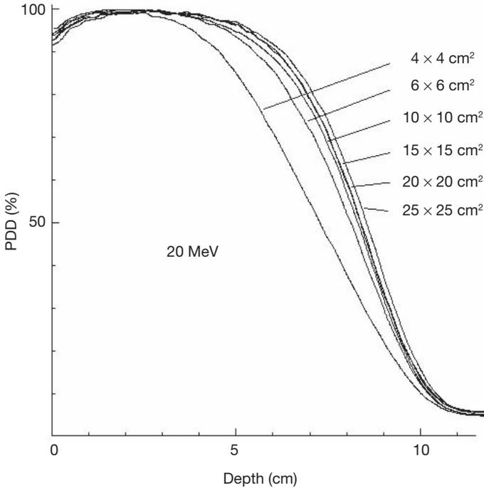
FIG. 8.4. PDD curves for different field sizes for a 20 MeV electron beam from a linac. It is clearly illustrated that for field sizes larger than the practical range of the electron beam ( $R_p$  is about 10 cm for this 20 MeV electron beam), the PDD curve remains essentially unchanged.
