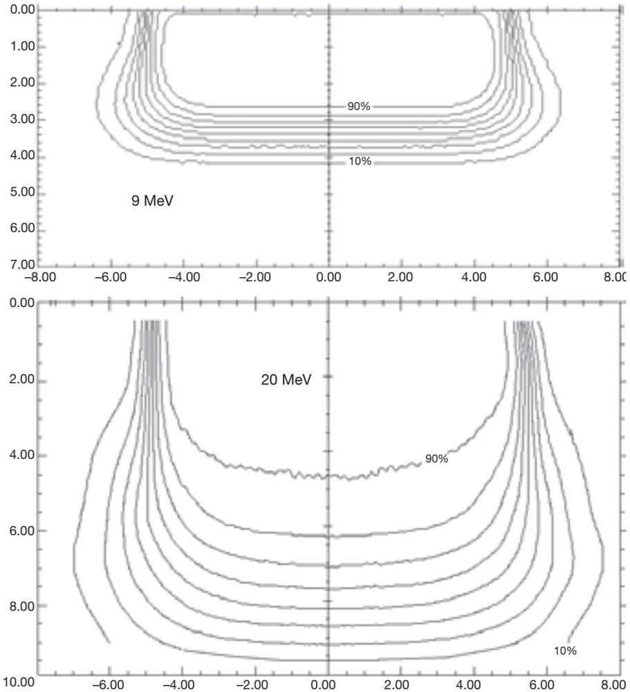
*FIG. 8.7. Measured isodose curves for 9 and 20 MeV electron beams. The field size is  $10 \times 10 \text{ cm}^2$  and  $SSD = 100 \text{ cm}$ . Note the bulging low value isodose lines for both beam energies. The 80% and 90% isodose lines for the 20 MeV beam exhibit a severe lateral constriction. The abscissa and the ordinate represent distance from the central axis and depth in a water phantom, respectively, measured in centimetres.*
