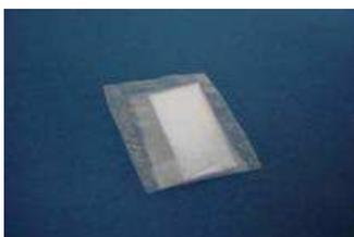
FIG.1. PVA bag containing ammonium bromide.
