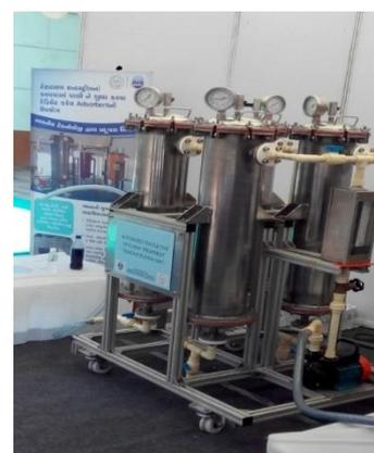
Fig. 2. Modular unit for treating Arsenic contaminated ground water (20,000 litres/day, 500ppb)
