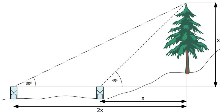
Figure 1: Placement of a rain collector to minimize the influence of nearby objects
