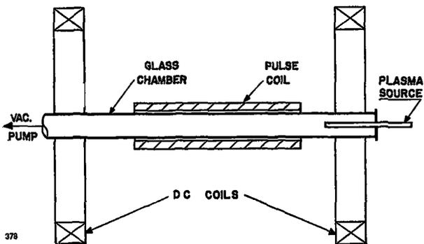
Figure 1. Schematic diagram and magnetic field distributions for System III
