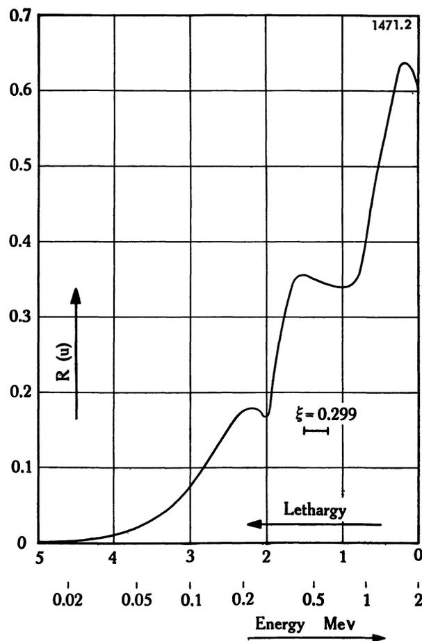
Figure 2. Reaction rate per unit lethargy, for pure Li<sup>6</sup>
