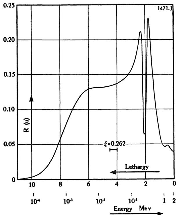
Figure 1. Reaction rate per unit lethargy, for natural lithium
