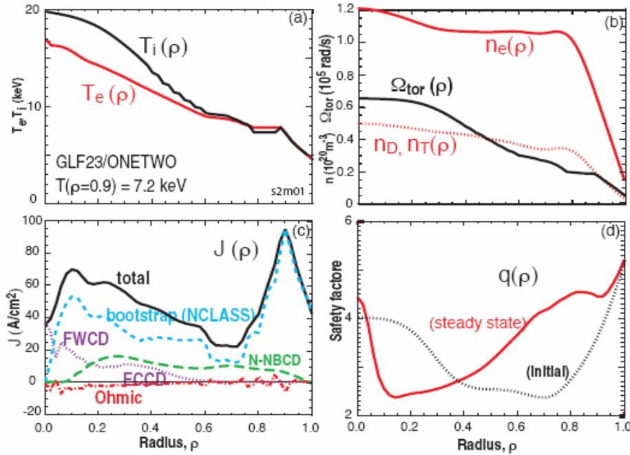
**Figure 3: The profiles for ITER steady-state scenario 4 [1] from the ONETWO code with the GLF23 transport model: a) temperatures, b) densities and toroidal rotation, c) current contributions, and d) the initial and final  $q$  profiles.**
