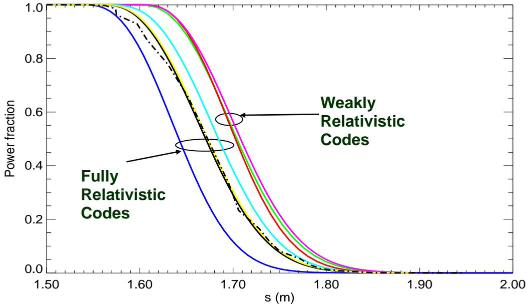
**Figure 1:** The fully relativistic codes (BANDIT-3D, CQL3D, GENRAY, OGRAY, and TORAY-GA) show slightly stronger absorption than the weakly relativistic codes (ECWGB, TORBEAM, and TORAY-FOM) for the ITER reference case at low density. The position of the 50% absorption fraction has a maximum variation of 7 cm, while the average difference between weakly and strongly relativistic models is ~4 cm.
