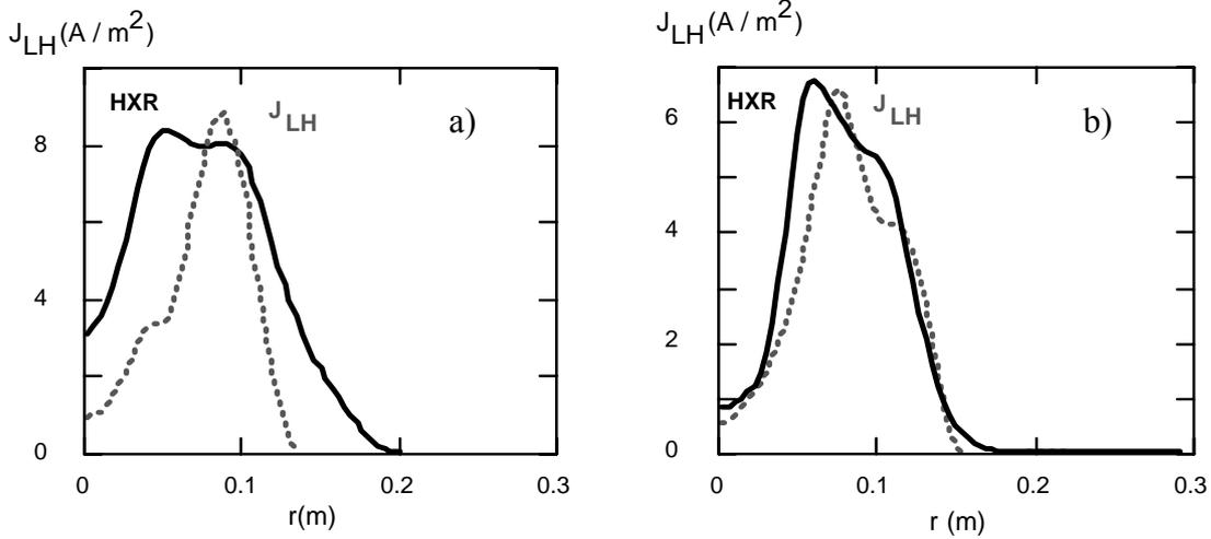
**Figure 2: HXR profile in FTU a) is broader than the calculated LH current profile, indicating possible diffusion of fast electrons that are not in the computed profile, while b) at higher density the agreement indicates that spatial diffusion is reduced. From ref [20].**
