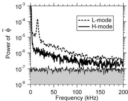
FIG.5 Comparison between the typical potential spectrum of L-mode and H-mode during NBH (HIBP).
