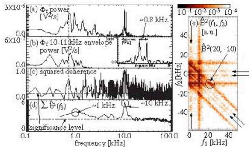
FIG.1 Potential spectrum and bicoherence measured by the RLP in the OH plasma. (Reprinted from Ref.11)
