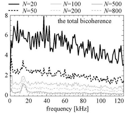
FIG.3 Convergence of the total bicoherence with realization number  $N$ .
