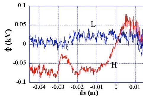
FIG.6 Potential profile measured by the HIBP during the ECH H-mode and ECH L-mode.  $I_p = 0.23\text{MA}$ ,  $B_{10} = 1.23\text{T}$ , ECR layer at  $0.86a$ ,  $P_{EC} = 0.37\text{MW}$ . Upper single null configuration.  $ds$  is a distance from the separatrix
