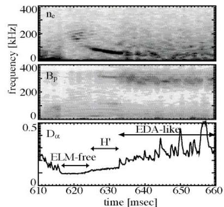
FIG.8 Density fluctuation by MRM (upper), magnetic fluctuation (middle) and  $D_\alpha$  signal (lower) in the H-mode by NBH. The electrostatic multi modes during the ELM free phase and the QCM during the H' phase are evident. (Reprinted from [23])
