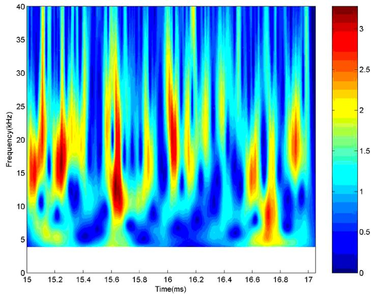
Fig. 5. Wavelet transform of potential fluctuations.
