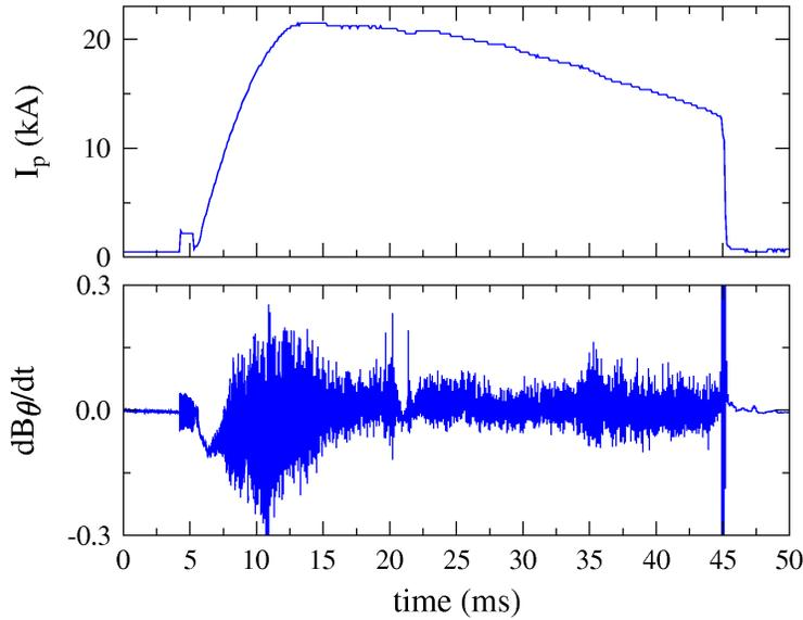
Fig. 6. The plasma current and a typical magnetic pickup coil signal. A compact torus is injected into the STOR-M discharge at  $t=20.1$  ms.
