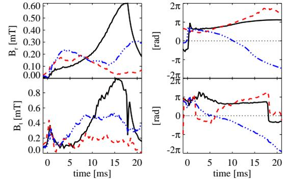
FIG. 7 Feedback using toroidal field sensors. Mode control scheme targeting  $m=1, n=-11$ . Variation of the complex feedback gain phase. Radial (top) and toroidal (bottom) field at wall. Left: Mode amplitudes, Right: Mode phases. Traces are shown for reference shot without feedback (full), feedback with complex gain phase  $\pi/2$  (dashed), feedback with gain phase  $5\pi/6$  (dot-dashed).
