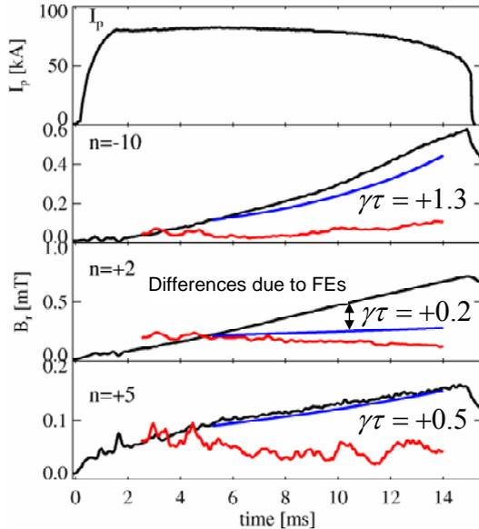
FIG. 8. The growth of three modes is analysed to determine the amplitude of the resonant field error. The black trace is the observed mode growth, the blue trace is the calculated growth from the amplitude at 5 ms and the known growth rate, and the red trace is the calculated field error amplitude based on Eq. (1)
