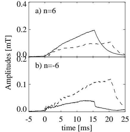
FIG. 4. The time dependence of mode harmonic amplitudes without feedback (solid line), with feedback using the 2x32 active coil configuration (dashed line); (a)  $|m|=1$ ,  $n=6$ . (b)  $|m|=1$ ,  $n=-6$ .
