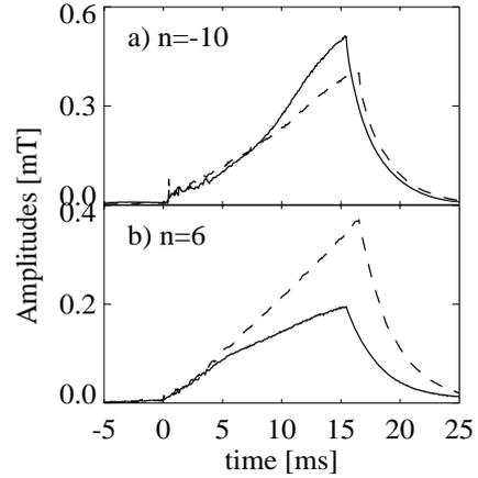
FIG. 2. The time dependence of mode harmonic amplitudes without feedback (solid line), with feedback using the 4x16 active coil configuration (dotted line); (a)  $m=1, n=-10$ . (b)  $m=1, n=6$ .
