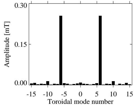
FIG. 3. The vacuum  $|m|=1$  mode spectrum for a targeted mode  $n=6$  for the active coil configuration with  $M_c=2$  and  $N_c=32$ .
