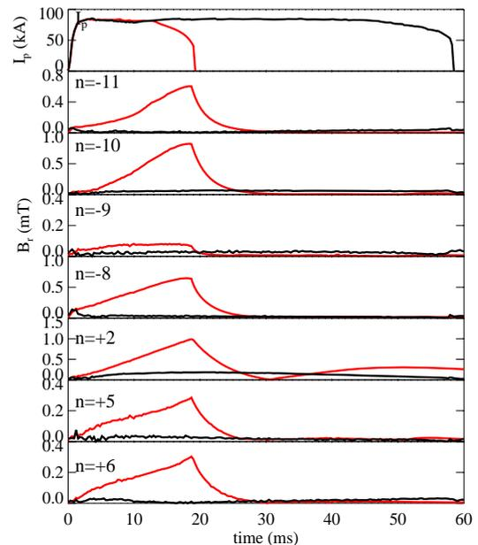
FIG. 5. Comparison of discharges with and w/o feedback control. The panels are as follows: plasma current, modes  $m=1$ ,  $n=-11$ ,  $-10$ ,  $-9$ ,  $-8$ ,  $+2$ ,  $+5$ ,  $+6$ .
