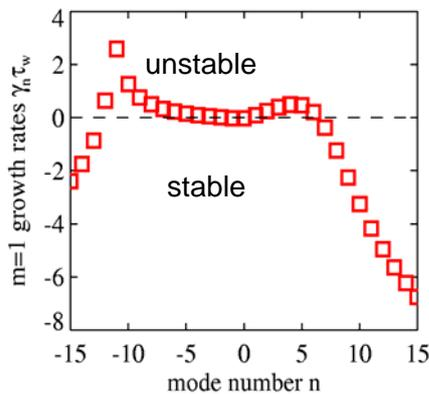
FIG.1. Spectrum of  $m=1$  modes in the EXTRAP T2R device. The unstable modes are  $-11 \leq n \leq -2$  (internally non-resonant) and  $1 \leq n \leq 6$  (externally non-resonant). Modes  $n \leq -12$  are resonant.
