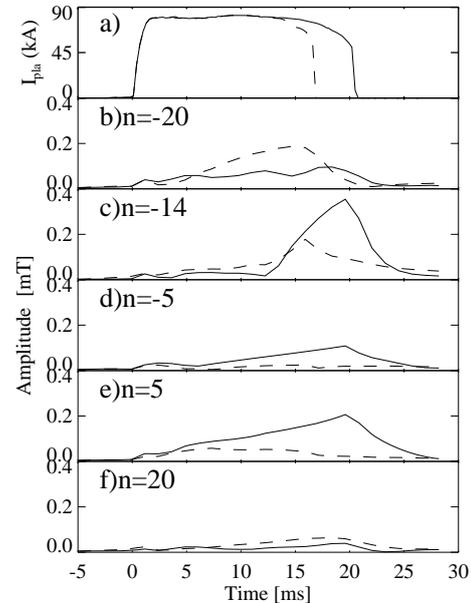
FIG. 6. Mode growth without feedback (solid line) and with fake rotating shell feedback (dashed line). (a) plasma current. (b)  $n=-20$ . (c)  $n=-14$ . (d)  $n=-5$ . (e)  $n=5$ . (f)  $n=20$ .
