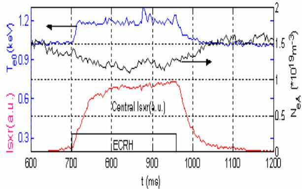
Fig.8. Basic parameters of on-axis ECRH experiment (central  $T_e$ , average  $N_e$ , central soft-X-ray).
