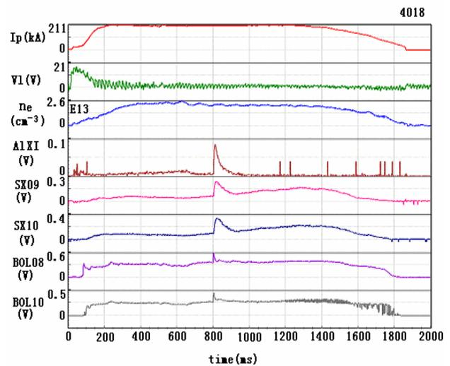
Fig.6. Time evolution of the plasma current, loop voltage and electron density, Al line brightness from VUV, the soft X-ray and bolometer signals.
