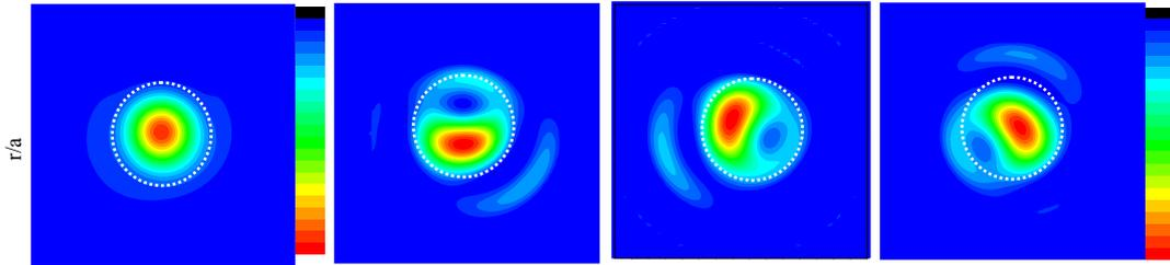
Fig.5 Four successive contour plots of the tomographically reconstructed soft x-ray emission measured every 0.01s after MBI. The white circle indicates the  $q=1$  surface.
