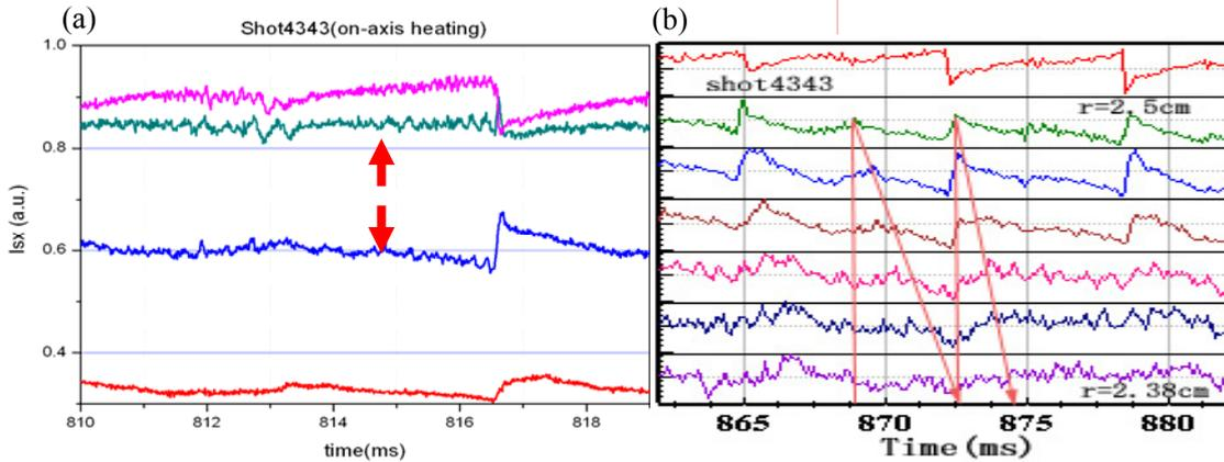
Fig.11 (a) A steep profile near the  $q=1$  surface before the compound crash; (b) the heat pulse propagation after the partial crash and main crash in a compound sawtooth cycle.
