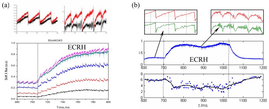
Fig.10 Destabilization of sawtooth by on-axis ECRH. A normal sawtooth becomes a compound sawtooth (a) or a saturated sawtooth (b).
