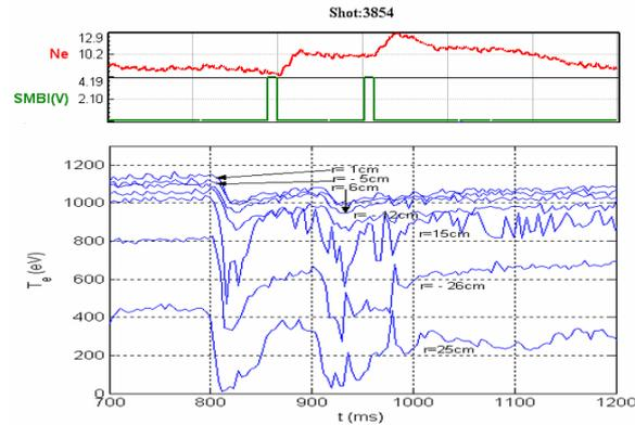
Fig.1 The plasma density increases  $2.2 \times 10^{19} \text{ m}^{-3}$  after MBI, while a temperature drop was observed in the central ECE channel.
