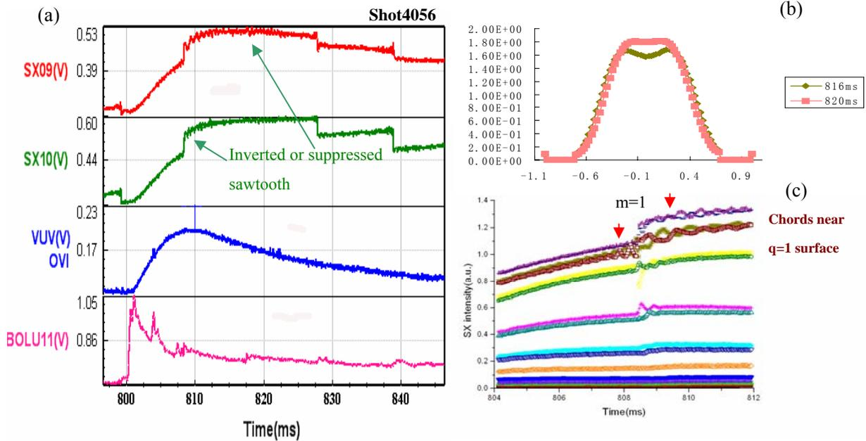
Fig.7. (a) Inverted sawteeth on the central Soft-X ray chords after impurity injection. (b) Profiles before and after the last inverted sawtooth crash. (c) The  $m=1$  oscillations on several central SX channels before and after the crash of an inverted sawtooth.
