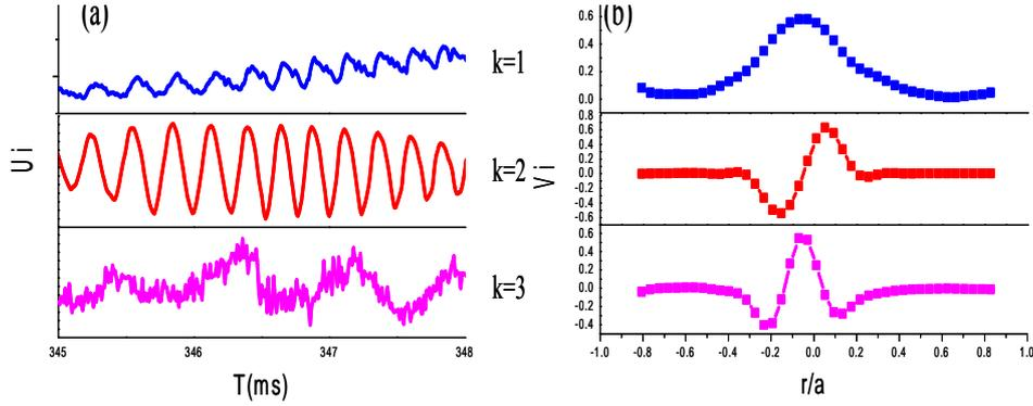
Fig.4 SVD analysis of signals: (a) time evolution of SVD principal components; (b) three corresponding spatial eigenfunctions. The  $k=2$  component describes a  $m=1$  perturbation, while the  $k=3$  component corresponds to a variation due to sawtoothing.
