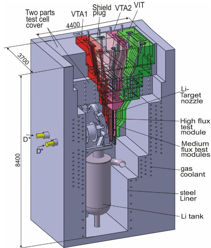
Fig. 1: Elevation view of the Target and Test Cell showing major components inside the cavity
