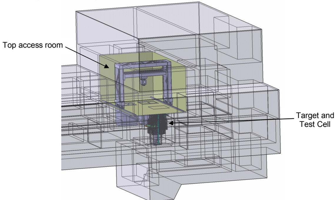
*Fig. 3: CATIA model showing part of the IFMIF main building with Target and Test Cell and top access room.*
