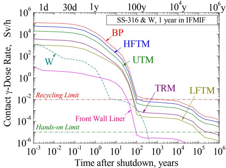
Fig. 4: Contact gamma dose rate after 1 year irradiation of several components in the Target and Test Cell, case of SS316 steel. BP target back-plate, W tungsten shifter, LFTM low flux test module, other abbreviations, see text.
