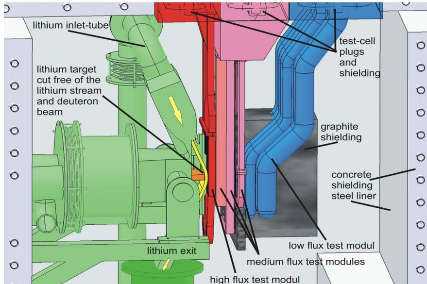
Fig. 2: Details of lithium target assembly and test module of the integrated CATIA model.
