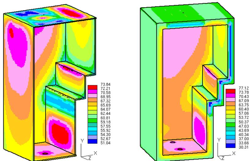
Fig. 7 Temperature (given in °C) of steel liner (left) and concrete wall (right) with helium atmosphere of 1 bar inside the Target and Test Cell cavity.
