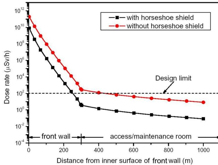
Fig. 5: Dose rate as a function of distance from the Target and Test Cell front wall (beam direction). A design variant with an additional shield encompassing the test modules (“horseshoe”) has been studied for comparison.
