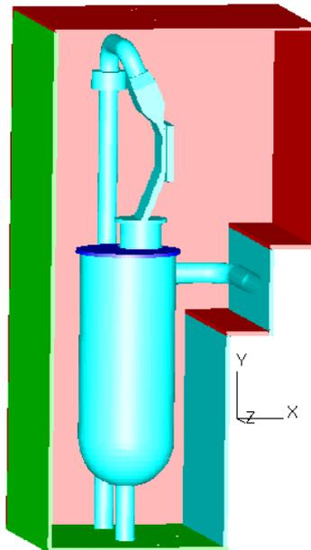
Fig. 6: Natural convection geometry model of the Target and Test Cell for STAR-CD.
