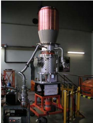
*Fig. 2. First Industrial 170 GHz, coaxial cavity gyrotron prototype*
