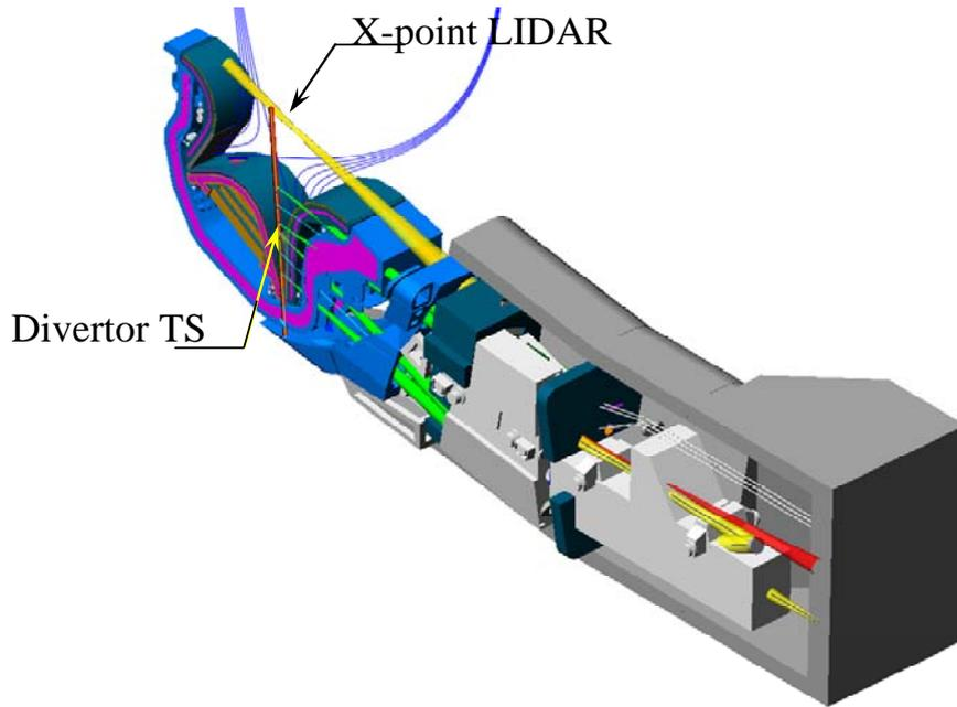
FIG. 6. Arrangement of the diagnostic racks shown as assembled in a divertor port and beam propagations in the regions near the X-point and outer divertor leg.
