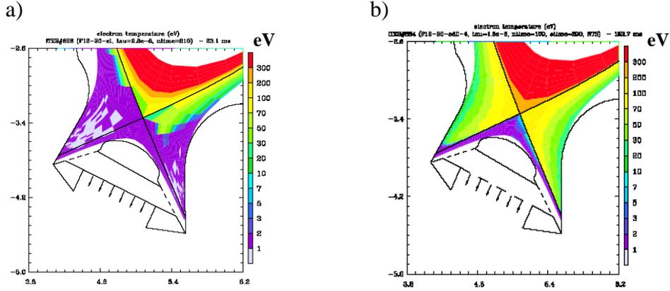
FIG. 5. 2D distribution of  $T_e$  in the divertor for two detachment scenarios. a) fully detached, b) partially detached.
