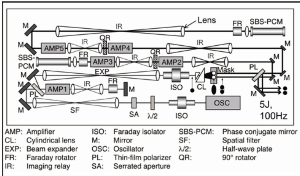
FIG.3. Laser optical design for edge Thomson scattering. High laser efficiency using Cr;Nd:YAG ceramic rods (efficiency is 2 times). Dual beam output to increase laser energy and to avoid laser damage.
