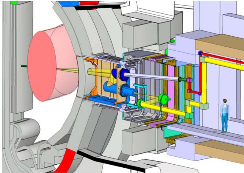
FIG. 1. Outline schematic of the port plug area LIDAR design for ITER.
