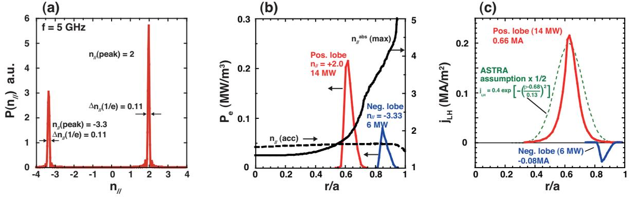
FIG. 2. (a) LH power spectrum vs  $n_{\parallel}$ . (b) Profiles of the absorption power to electrons from the positive and negative lobes of the LH power spectrum (a). Also shown are a rough estimate of the maximum  $n_{\parallel}$  for absorption  $n_{\parallel}^{\text{abs}}(\text{max}) = 6.5/T_e^{0.5}$  [14] and the accessibility condition for the plasma. (c) LHCD profiles for the forward and reverse power, and the assumed profile in the previous simulation (1/2 scale).
