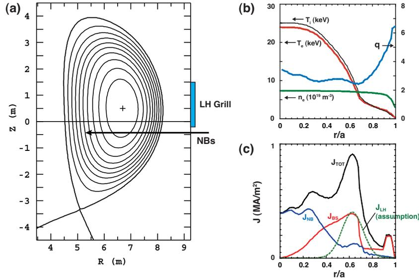
FIG. 1. The reference ITER scenario 4 [4] : (a) Equilibrium and the LH launcher position. Also shown is the poloidal projection of the off-axis NB injection used in the NBCD code benchmark. (b) The radial profiles of the temperatures, electron density and safety factor, and (c) the total current density ( $J_{\text{TOT}}$ ) and contributions from NBCD ( $J_{\text{NB}}$ ), the bootstrap current ( $J_{\text{BS}}$ ) and LHCD ( $J_{\text{LH}}$ ).
