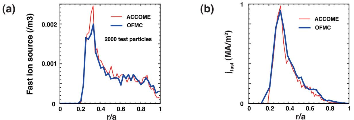
FIG. 4. (a) The reference scenario 4 equilibrium and poloidal projection of the off-axis NB injection. Profiles of (b) the fast ion source and (c) the fast ion current density (toroidal) calculated with ACCOME and OFMC.
