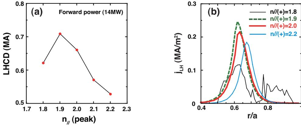
FIG. 3. (a) Peak  $n_{\parallel}(+)$  dependence of the LHCD for a forward LH power 14 MW. (b) LHCD profiles for peak  $n_{\parallel}(+) = 1.8, 1.9, 2.0$  and  $2.2$ .
