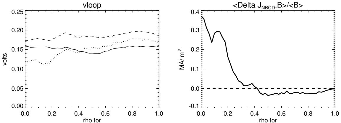
Figure 6: *Left plot: Loop voltage profiles calculated before (solid), 100 ms after (dotted) and 150 ms after (dashed curve) the substitution of 5MW of off-axis NBI heating by 5MW on-axis heating for #19026 ( $I_p = 0.8$ MA,  $B_t = 2.5$ T). Right plot: Change in the NBCD profile inferred from the difference in the solid and dotted loop voltage profiles.*
