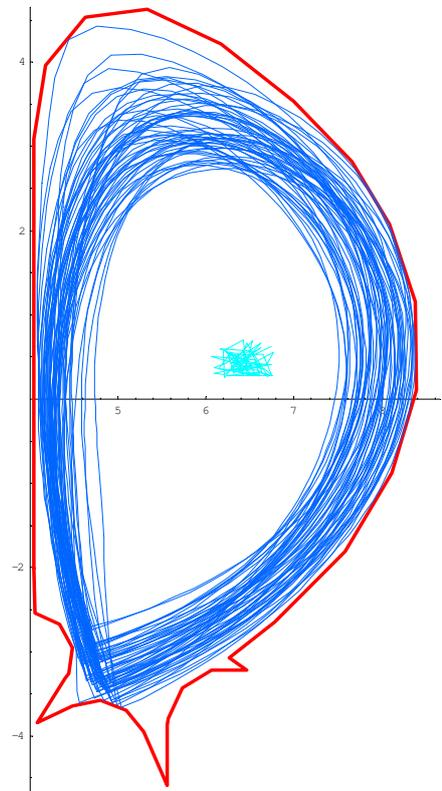
Figure 1: *ITER first wall and 60 randomly chosen separatrix contours with corresponding magnetic axis locations.*
