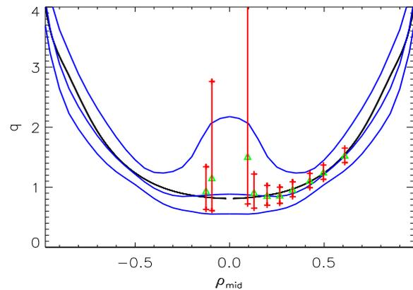
Figure 4: *FPJ q-profiles with 95% confidence bands from equilibrium database analysis (blue curves) for #12036,  $t=2.0$  s. The black curve is the CLISTE reconstruction. “Experimental”  $q$ -values and error bars are shown as green triangles and red lines, respectively (see text).*
