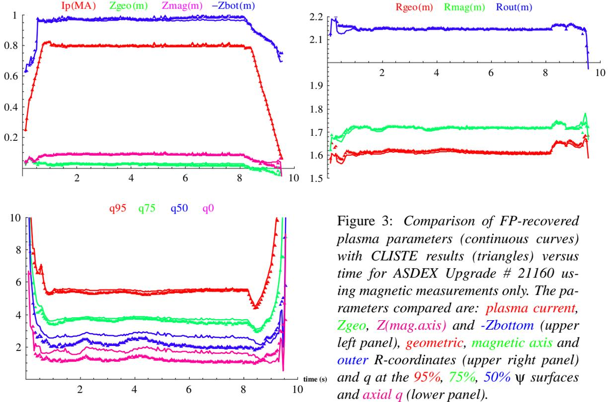
Figure 3: Comparison of FP-recovered plasma parameters (continuous curves) with CLISTE results (triangles) versus time for ASDEX Upgrade # 21160 using magnetic measurements only. The parameters compared are: plasma current,  $Z_{geo}$ ,  $Z(\text{mag.axis})$  and  $-Z_{bottom}$  (upper left panel), geometric, magnetic axis and outer  $R$ -coordinates (upper right panel) and  $q$  at the 95%, 75%, 50%  $\psi$  surfaces and axial  $q$  (lower panel).
