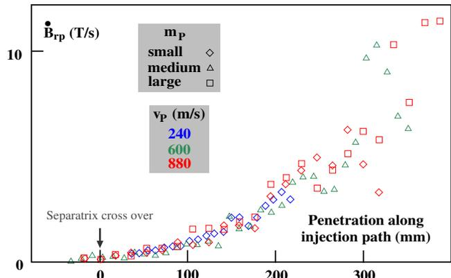
FIG. 2: Pellet induced MHD perturbation in AUG versus pellet position along the injection path, separatrix position defines 0. At the same position in the plasma, the same magnitude for the pellet driven MHD response is observed for any pellet speed and/or mass applied.
