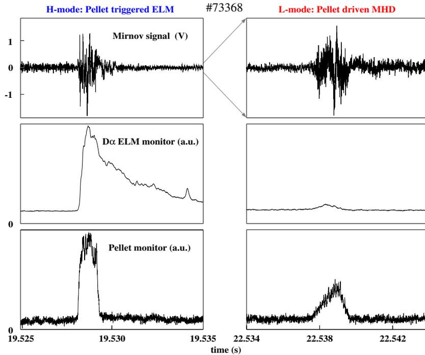
FIG. 4: Mirnov coil response, divertor  $D_\alpha$  ELM monitor and pellet ablation (top to bottom) for pellets in JET (accompanied possibly by debris) triggering an ELM during an H-mode phase (left) but driving only transient MHD activity declining after burn out (right, note expanded y-scale of upper box).
