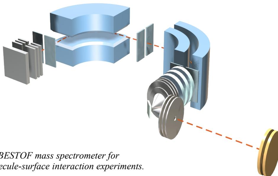
*Fig. 1: BESTOF mass spectrometer for ion/molecule-surface interaction experiments.*
