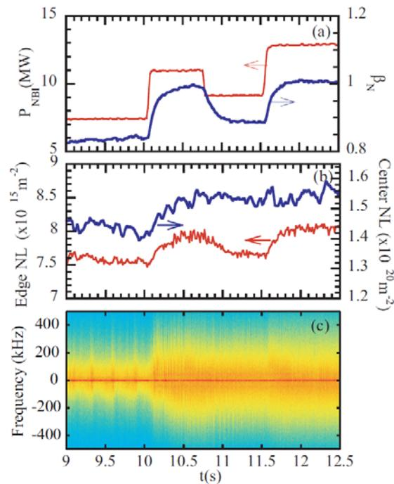
Fig.4 Time history of (a) NB power, notmalized beta ( $\beta_N$ ), (b) line integrated density and (c)reflected power spectrum in JT-60U.
