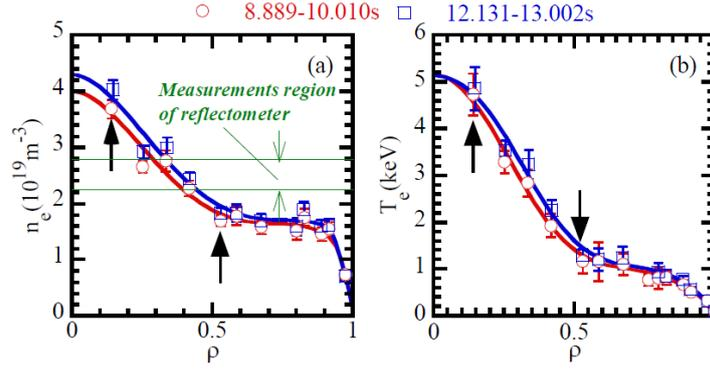
Fig.5 (a)  $n_e$  and (b)  $T_e$  profile at low (7.4MW,  $t=8.889-10.010s$ ) and high (12.9MW,  $t=12.131-13.002s$ ) NB power. Black arrows indicate YAG Thomson points when core scale length was calculated.
