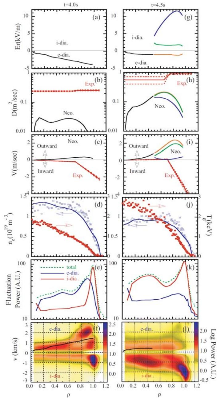
Fig.9(a), (g) Radial profile of  $E_r$ , (b), (h)  $D$ , (c),(i)  $V$ , (d),(j)  $n_e$ ,  $T_e$ , (e), (k) fluctuation power and (f), (l) fluctuation phase velocity. (a)-(f) are at low NB power (1.1MW at  $t = 4.0s$ ) and (g)-(l) are at high NB power (5.6MW at  $t = 4.5s$ ). Neoclassical  $E_r \times B_t$  rotation velocities are indicated by black lines in Fig.9 (f) and (l).
