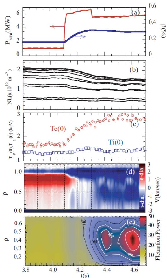
Fig.8 Time history of (a) NB heating power, diamagnetic  $\beta$ , and (b) line integrated density. Higher values (upper trace) correspond to the chord close to magnetic axis. (c) central electron and ion temperature, (d) fluctuation phase velocity and (e) fluctuation power at  $\rho=0-0.7$ .  $R_{\text{ax}}=3.6\text{m}$ ,  $B_t=2.75\text{T}$ . In Fig.8(d), red and blue colors indicate electron and ion diamagnetic directions in laboratory frame, respectively.
