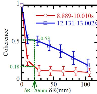
Fig.6 Radial coherence profile at high (7.4MW,  $t=8.889-10.010s$ ) and low (12.9MW,  $t=12.131-13.002s$ ) NB power.  $\delta R$  is the radial distance between the fixed and scanned channels.
