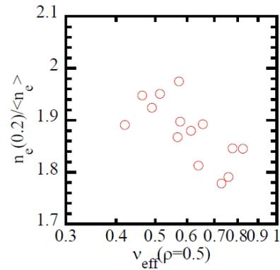
Fig.3 The dependence of the density peaking factor on  $\nu_{eff}$  from JT-60U 2008 campaign. The data is from 14 cases of 5 discharges.
