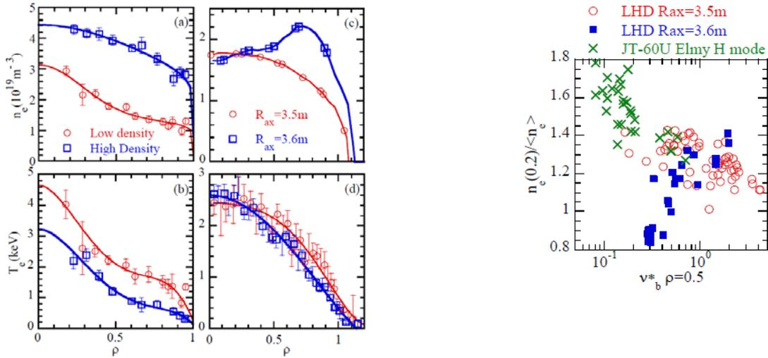
Fig. 1 (a), (c)  $n_e$ , and (b),(d)  $T_e$  profiles. (a) and (b) from JT-60U, and (c) and (d) from LHD. Here, plasmas in low and high density plasmas in JT-60U, and those at  $R_{ax}=3.5$  m and  $R_{ax}=3.6$  m in LHD are compared.
