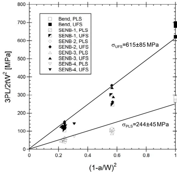
FIG. 4. Notch Sensitivity of pilot-grade NITE-SiC/SiC composites.
