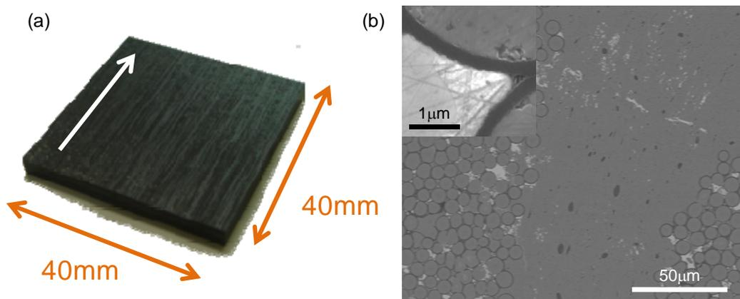
FIG. 1. (a) Outlook and (b) typical microstructures of pilot-grade NITE-SiC/SiC composites.
