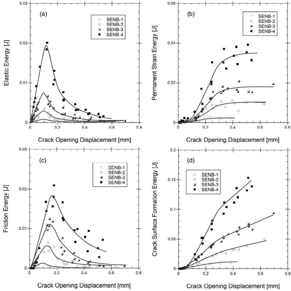
FIG. 6. Crack surface formation energy vs. crack opening displacement.
