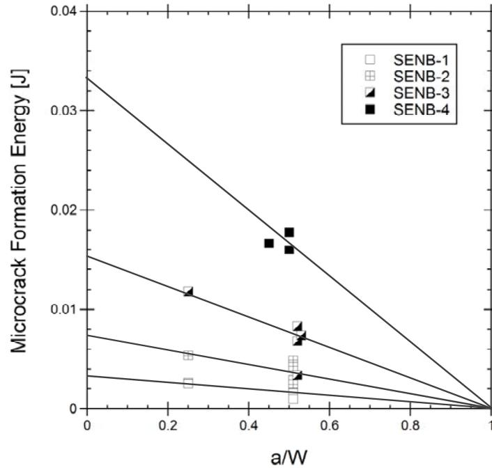
FIG. 7. Micro-crack formation energy vs. initial notch depth.
