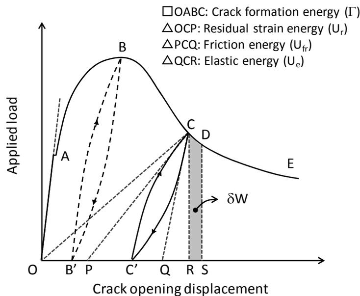
FIG. 5. Schematic illustration of load-crack opening displacement curve.
