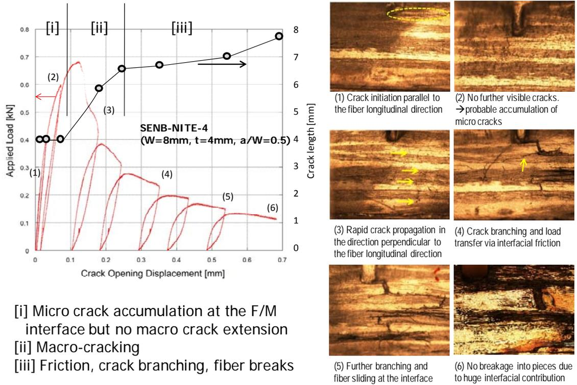
FIG. 3. Typical SENB behavior of pilot-grade NITE-SiC/SiC composites.
