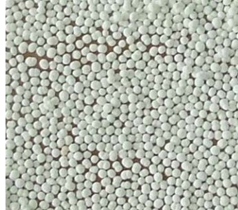
Fig.13 \text{Li}_4\text{SiO}_4 pebbles of diameter 1mm
