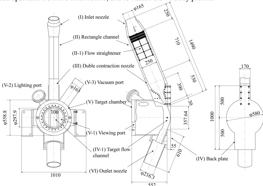
FIG.2. Structure of the integrated TA
