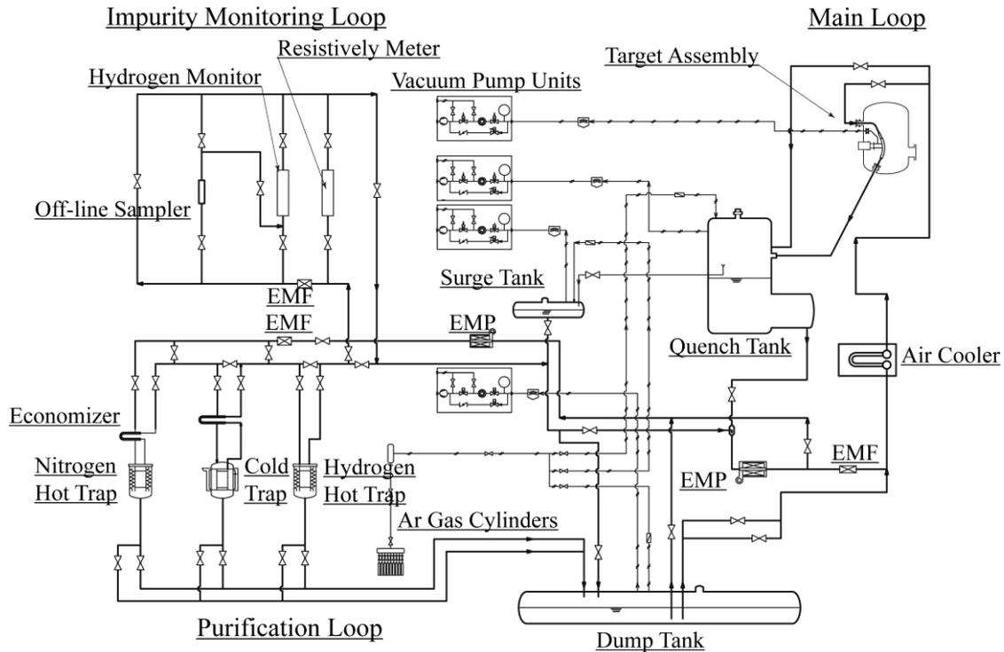
FIG.1. Pipe and instruments diagram of the ELTL
