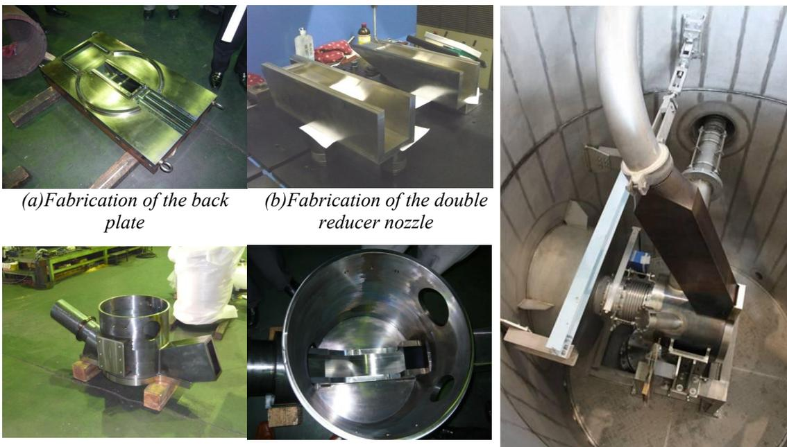
(c) Assembly of the back plate, the double contraction nozzle, the outlet nozzle and the target chamber
