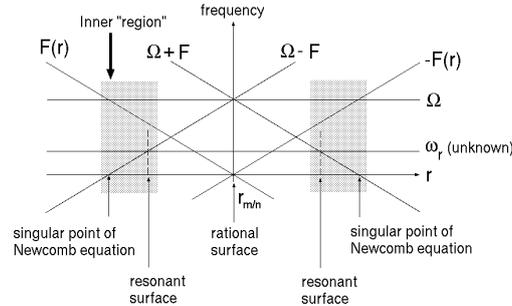
FIG. 1. Schematic view of locations of the rational surface, the singular points of the generalized Newcomb equation and the resonant surface for the shear Alfvén waves. The singular points split from the rational surface due to the Doppler shift. The resonant surface deviates from the singular points since the unstable mode has a finite real frequency in rotating plasmas.
