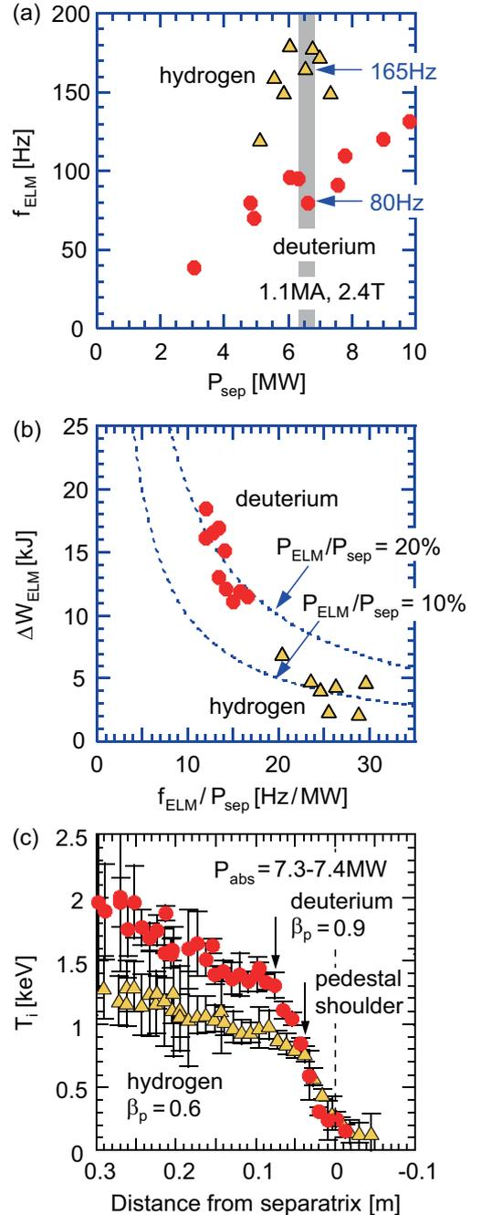
FIG. 6: (a) Dependence of  $f_{\text{ELM}}$  on  $P_{\text{sep}}$  for hydrogen and deuterium plasmas. (b) Relation between  $\Delta W_{\text{ELM}}$  and  $f_{\text{ELM}}/P_{\text{sep}}$ . (c) Edge  $T_i$  profiles at  $P_{\text{sep}}$  of 7.3–7.4MW.
