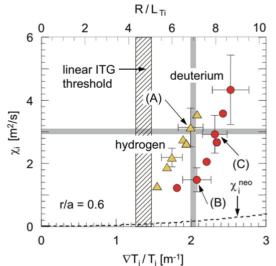
FIG. 5: Relationship between  $\chi_i$  and  $\nabla T_i/T_i$  (or  $R/L_{T_i}$ ) evaluated at  $r/a = 0.6$ .
