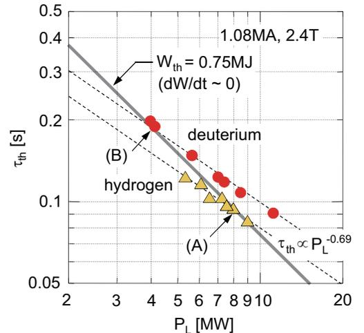
FIG. 1: Dependence of the thermal energy confinement time  $\tau_{\text{th}}$  on the loss power  $P_L$  for deuterium and hydrogen H-mode plasmas performed at 1.08MA and 2.4T. A pair of plasmas with  $W_{\text{th}} (= P_L \tau_{\text{th}})$  of 0.75MJ are indicated as (A) and (B).
