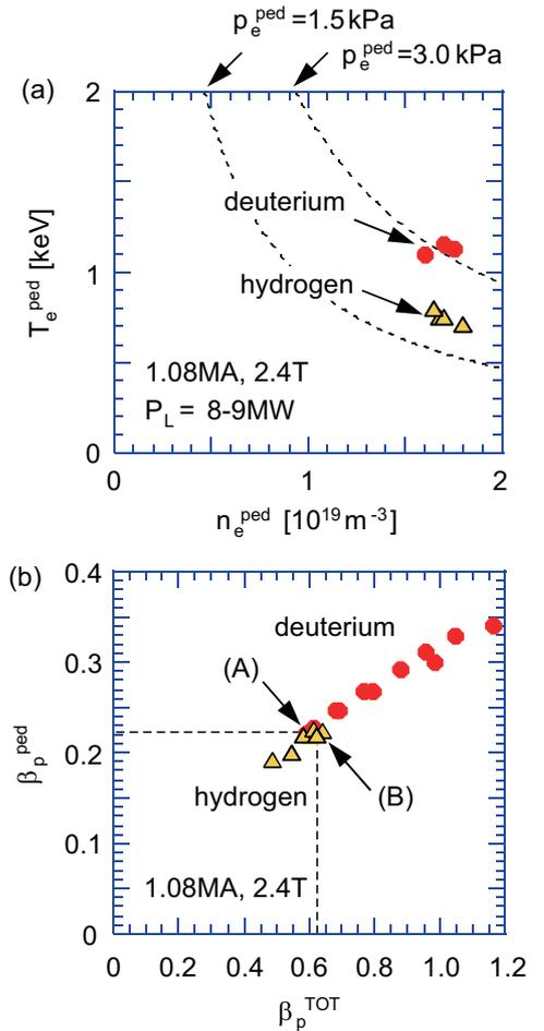
FIG. 7: (a) The relationship between  $n_e^{\text{ped}}$  and  $T_e^{\text{ped}}$  at  $P_L$  of 8 – 9MW for hydrogen and deuterium H-mode plasmas. (b) The relationship between  $\beta_p^{\text{TOT}}$  and  $\beta_p^{\text{ped}}$ .
