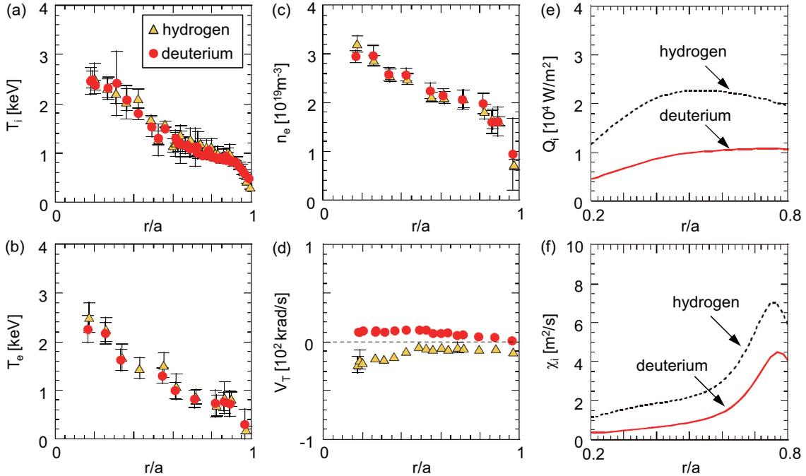
FIG. 2: Profiles of  $T_i$ ,  $T_e$ ,  $n_e$ ,  $V_T$ ,  $Q_i$ , and  $\chi_i$  which correspond to the hydrogen and deuterium discharges with the same  $W_{\text{th}}$  of 0.75MJ.
