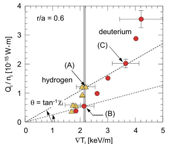
FIG. 3: Relationship between  $Q_i/n_i$  and  $\nabla T_i$  evaluated at  $r/a = 0.6$ . The data for hydrogen and deuterium with the same  $W_{\text{th}}$  of 0.75MJ are indicated as (A) and (B), respectively.
