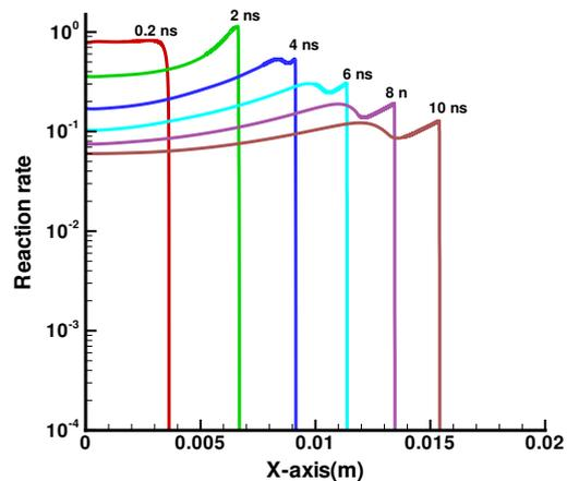
Fig. 4. Reaction rates (to be multiplied by  $10^{36} \text{ m}^{-3} \text{ s}^{-1}$ ) in solid DT at 1 ps pulse of energy flux  $E^* = 3 \times 10^8 \text{ J/cm}^2$  KrF laser irradiation depending on the fuel depth  $x$  at different times up to 10 ns.
