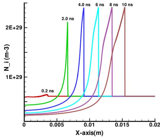
Fig. 1. Ion densities  $N_i$  depending of the depth  $X$  after a one ps  $3 \times 10^8 \text{ J/cm}^2$  laser pulse of 248 nm wave length has irradiated solid density DT. Parameter is the time after the ps interaction
