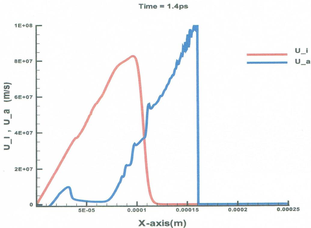
Fig. 5. Irradiation of a 0.5 ps 248 nm wave length long laser pulse of  $10^{21}\text{ W/cm}^2$  on solid DT. Ion velocity  $U_i$  and velocity of the alpha particle fluid depending on depth  $X$  in the target at time 1.4 ps.
