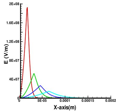
Fig. 3. Longitudinal electric field  $E$  as in case of Fig. 1 for  $E^* = 10^8 \text{ J/cm}^2$  depending of the depth  $X$  at times of 40ps; 400ps; 1ns; 2 ns from the highest maximum respectively.
