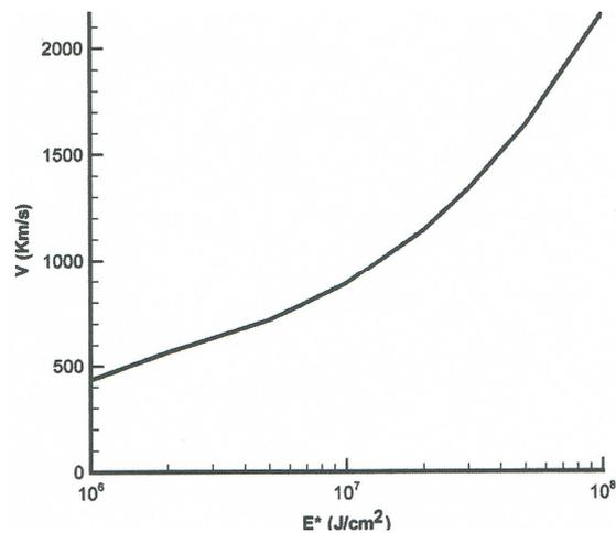
Fig. 2. Velocity  $V$  of the fusion flame at 2 nanoseconds after the initiating ps laser pulse of 248 nm wavelength depending on the energy flux  $E^*$ .
