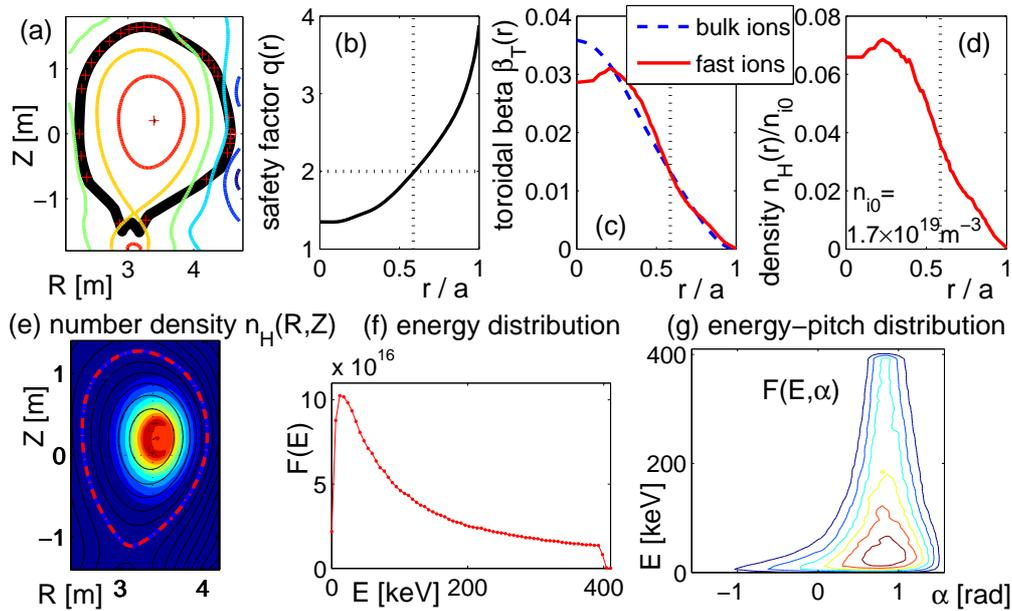
FIG. 1: JT-60U plasma in shot E039672 before the onset of an ALE. Panel (a) shows shape of magnetic surfaces and the wall, (b-d) the profiles of safety factor, bulk ions and fast ions, and (e-g) the phase-space distribution of fast ions computed by F3D-OFMC.
