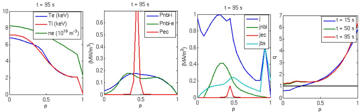
**Fig. 7:** METIS simulations of Scenario 4-2 (advanced inductive). From left to right: temperature and density profiles at  $t = 95$ s; power deposition profiles (NBI power to ions and to electrons, EC power); current density profiles; safety factor profile evolution.
