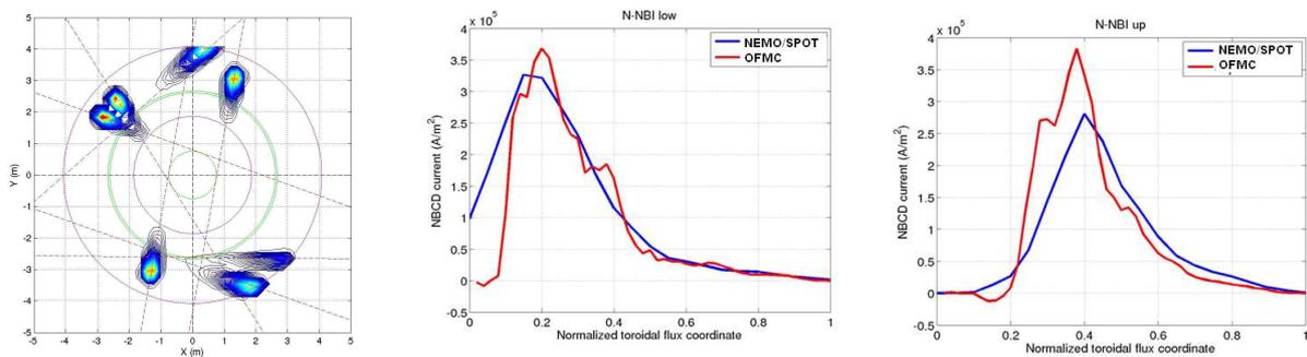
**Fig. 1 :** Left : toroidal view of the power deposition profiles of the JT-60SA injected Neutral Beams, computed by means of the NEMO/SPOT code. Middle : driven current profiles computed by NEMO/SPOT and by F3D-OFMC for the lower Negative neutral beam ; right : the same for the upper beam.
