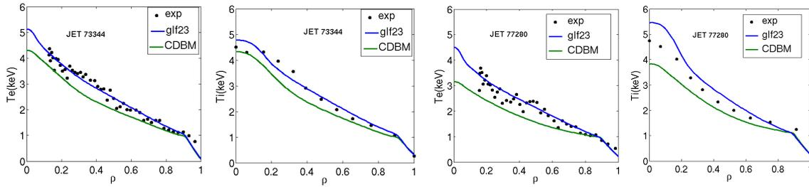
**Fig. 5:** Comparison between the electron and ion temperatures profiles obtained by CRONOS with GLF23 and modified CDBM transport models for shots 73344 and 77280.
