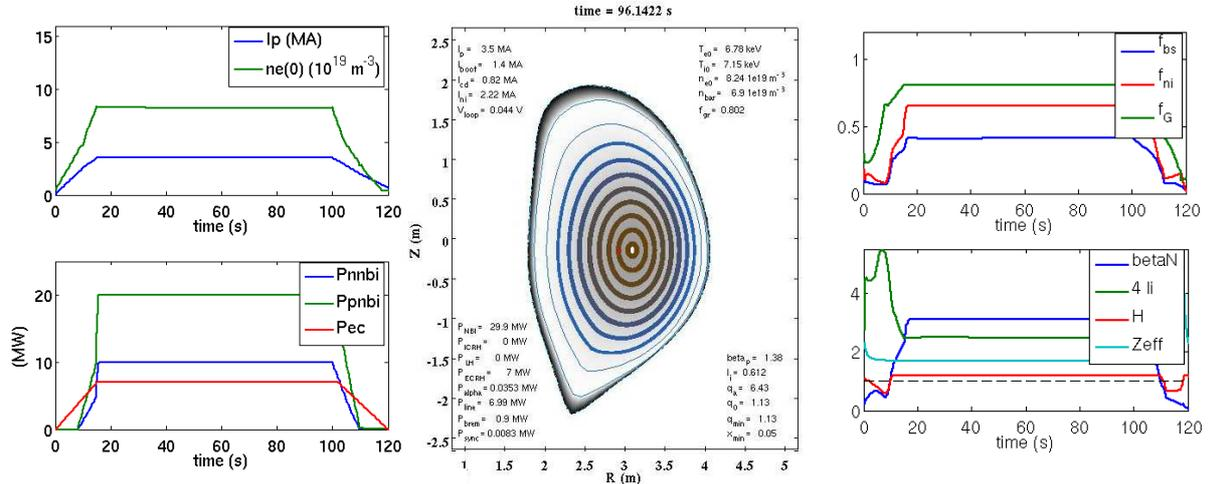
**Fig. 6:** METIS simulations of Scenario 4-2 (advanced inductive). Time evolution of plasma current and central electron density (top left); time evolution of heating powers - positive NBI, negative NBI and ECRH (bottom left); magnetic equilibrium at the end of the flat-top phase (middle). Time evolution of bootstrap, non-inductive and Greenwald fractions (top right); time evolution of  $\beta_N$ ,  $4I_i$ , H factor and  $Z_{eff}$  (bottom right).
