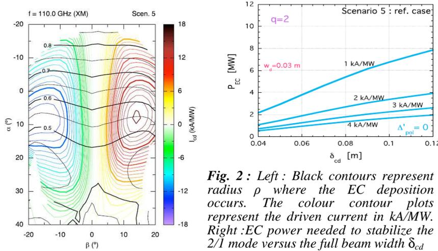
**Fig. 2 :** Left : Black contours represent radius  $\rho$  where the EC deposition occurs. The colour contour plots represent the driven current in kA/MW. Right : EC power needed to stabilize the 2/1 mode versus the full beam width  $\delta_{cd}$
