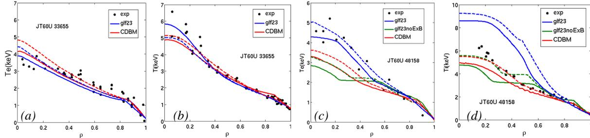
**Fig. 4:** Comparison between the electron (a,c) and ion (b,d) temperatures profiles with those obtained with CRONOS (solid) and TOPICS (dashed) with GLF23 and CDBM transport models for shot 33655 and 48158.
