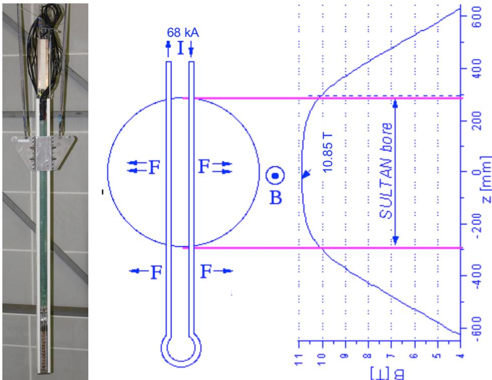
FIG. 1. An assembled TF conductor sample and the test geometry in SULTAN.
