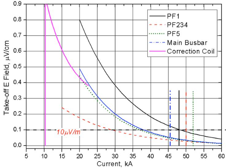
FIG. 3. Take-off voltage vs current for the NbTi ITER CICC.
