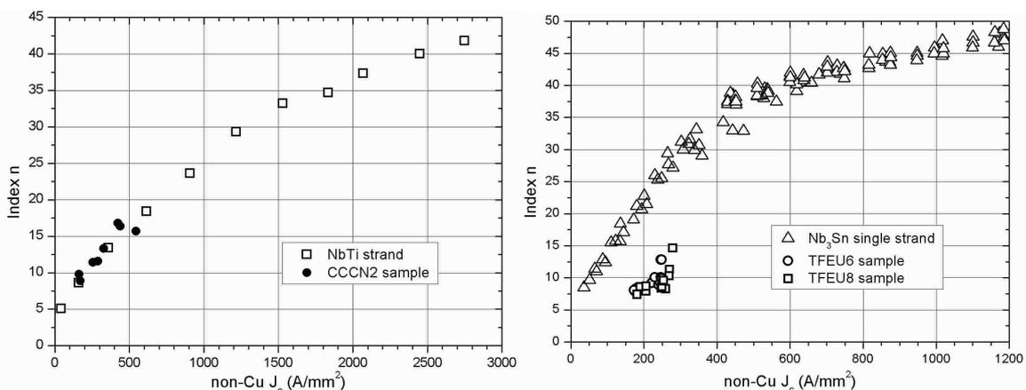
FIG. 2. Comparison of  $n$ -index for strand and CICC:  $NbTi$  (left) and  $Nb_3Sn$  (right).
