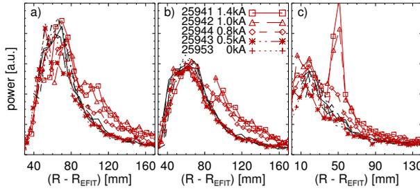
FIG. 3: Comparison of heat flux profiles measured by the divertor probes for varying perturbation coil current in even parity,  $60^\circ$  configuration. a), b) upper sectors, c) lower sector. Black lines without symbols: time window before  $t = 0.22$  s, red lines with symbols: time window after  $t = 0.22$  s.
