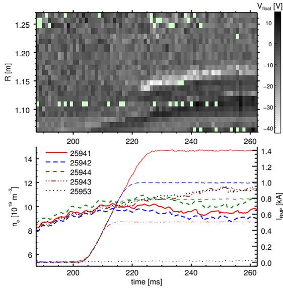
FIG. 1: Time dependence of  $V_{float}$  in even parity  $60^\circ$  phase shot 25941 (top) and the RMP coil current and electron density evolution in a series of shots in the same RMP coil configuration (bottom). The green points in the top graph represent unavailable data.
