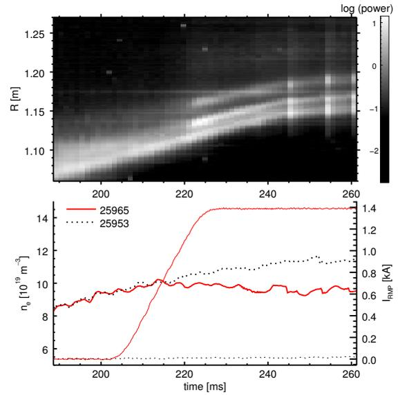
FIG. 2: Time dependence of the profile of the logarithm of the heat flux calculated from the IR camera data in even parity  $0^\circ$  phase shot 25965 (top) and the RMP coil current and electron density evolution in this shot compared with a reference shot (bottom).
