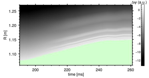
FIG. 4: Time evolution of the radial distance to the perturbed outboard midplane separatrix, mapped to the divertor, using the conditions in shot 25965.
