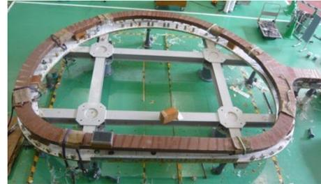
*Fig. 3 1/3 scale prototype of TF winding pack manufactured by JA*
