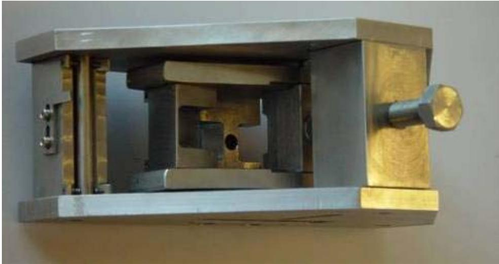
*FIG. 18. 4-point bending device for round robin exercise no. 1*
