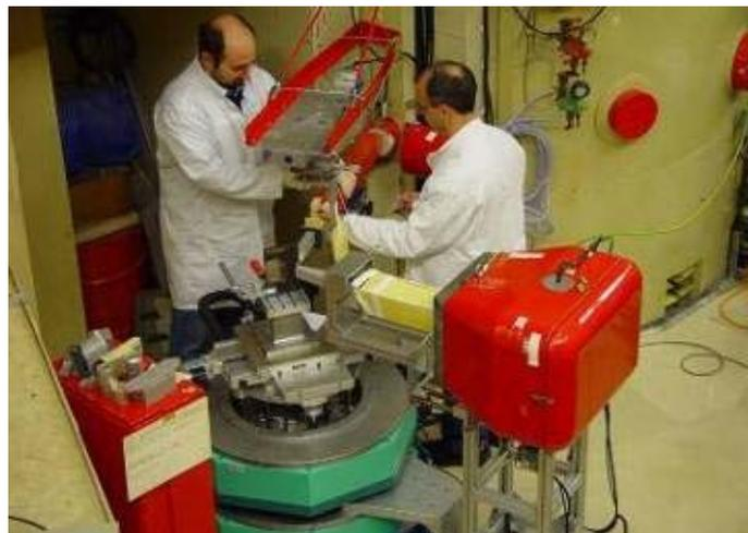
*FIG. 1 Setting up the new diffractometer at HFR beam tube HB5*
