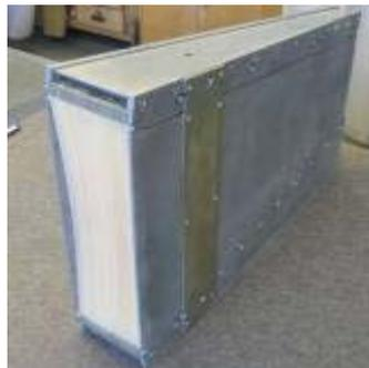
FIG. 13. Multi-slit radial collimator with 10-degree acceptance angle is manufactured for FSD.
