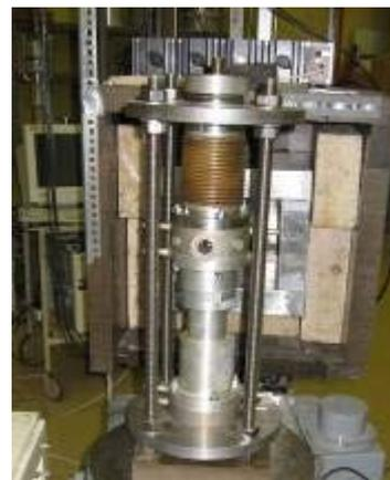
FIG. 10. The tensile test with combined furnace.
