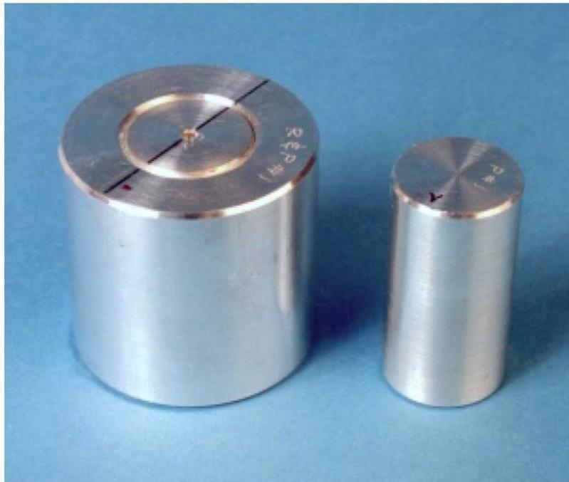
*FIG. 19. Aluminium shrink fit Ring & Plug specimens for round robin exercise no. 2*
