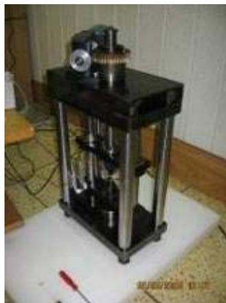
FIG. 14. New deformation (tensile/compressive) machine is to be installed at FSD.
