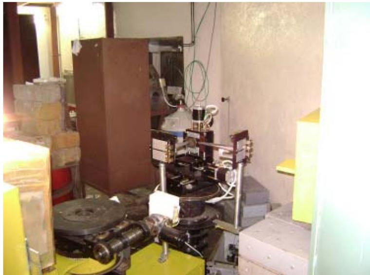
*FIG. 7. Residual stress diffractometer at Pitesti.*
