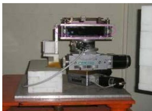
FIG. 16. Monochromator bending device
