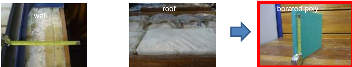
Fig.4. Improvements in the shielding
