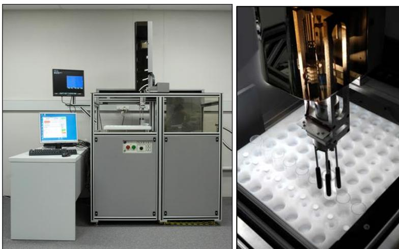
There are two ORTEC HPGe detectors (27% and 32% relative efficiency). The software packages used for data accumulation and analysis are ORTEC Maestro, HyperLab and Kayzero for Windows.
