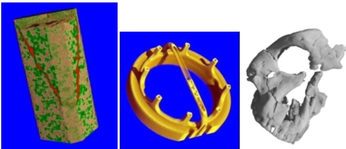
**Fig. 6.5.3:** Neutron tomograms obtained at SANRAD facility: left - thin sectioning of geological sample with different minerals pseudo colored, middle - helicopter component with blockage in oil pipe, right - reconstruction of a fossil.
