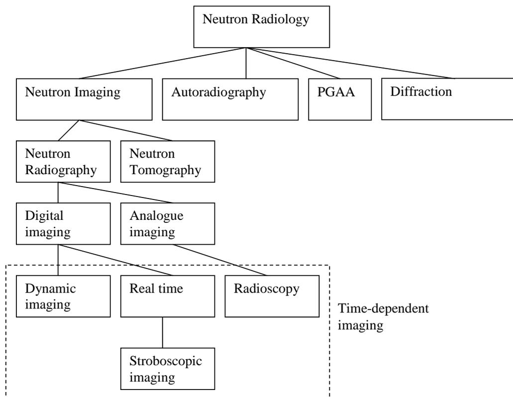
**Fig. 5.2.1:** A Relation between the different aspects and methods in neutron imaging.
