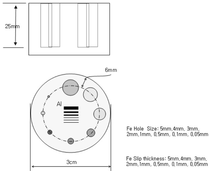
**Resolution Phantom (holes and slips)**
