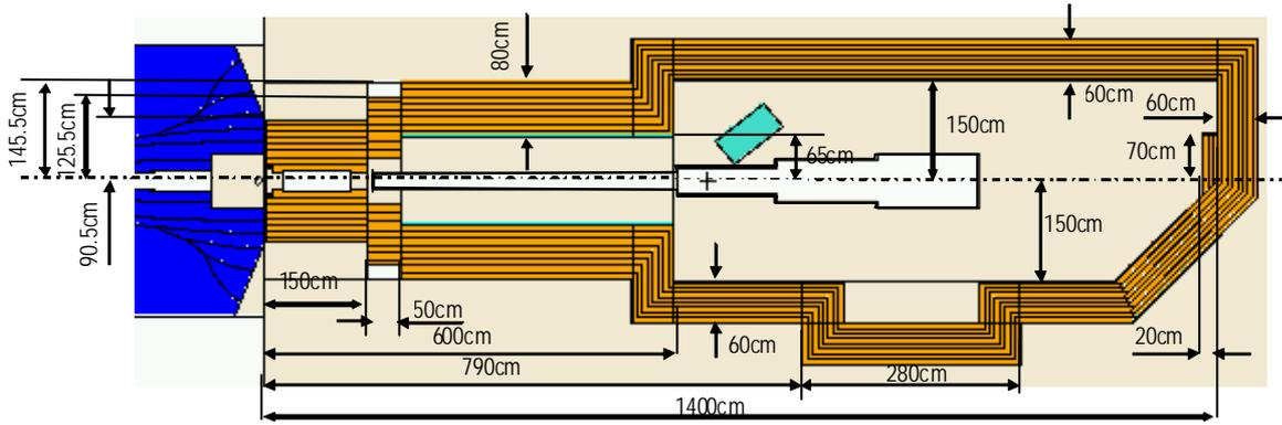
**Fig. 6.5.2:** A schematic diagram (top view) of the new SANRAD facility.
