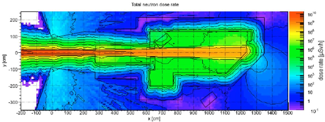
**Fig. 6.5.2:** Simulated dose rate distribution of the new SANRAD facility using the MCNPX code (also see Fig. 6.4.2).
