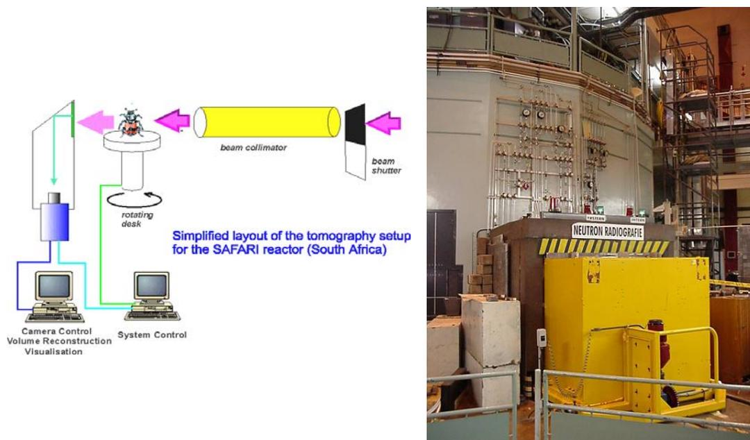
**Fig. 6.5.1:** *Left - Simplified layout of the tomography setup for the SAFARI reactor (South Africa), Right - Photo of the facility.*
