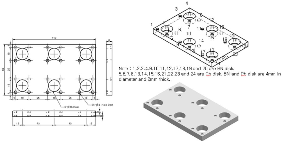
Digital Image Quality Measurement Polyethylene Block
