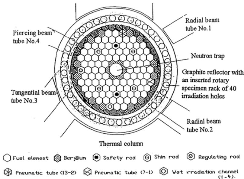
**Fig. 1.** Cross section of the reactor core.
