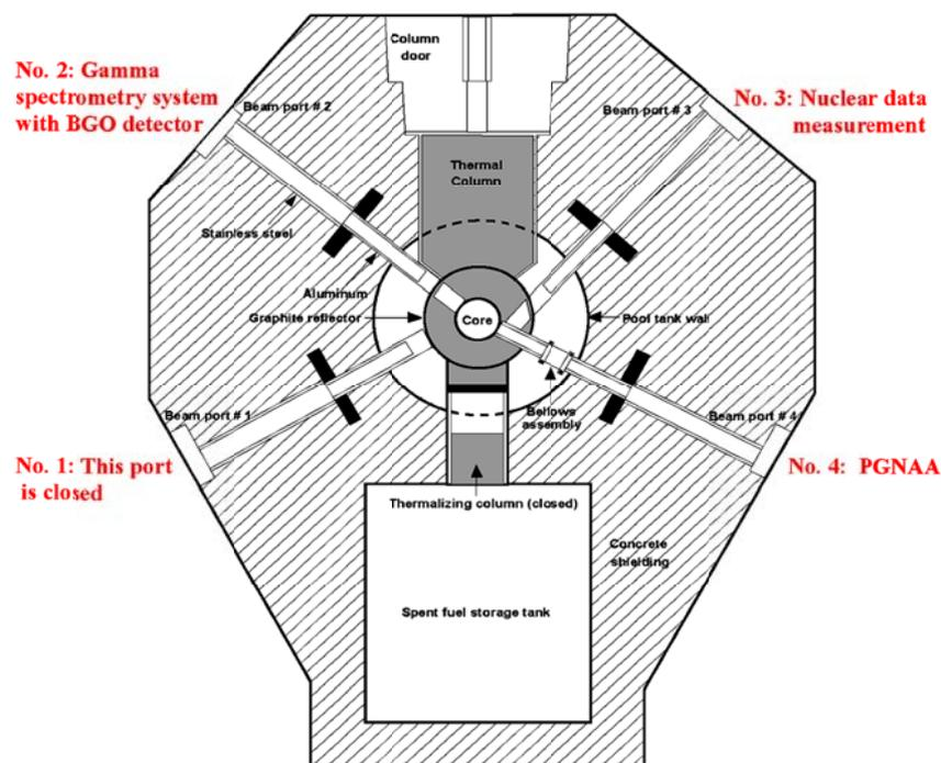
Fig. 4. Horizontal section view of the Dalat Nuclear Research Reactor.
